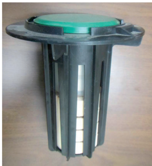
Fig. 2. Station with inspection cartridge with cellulose tablets and a monitoring base made of southern yellow pine.
