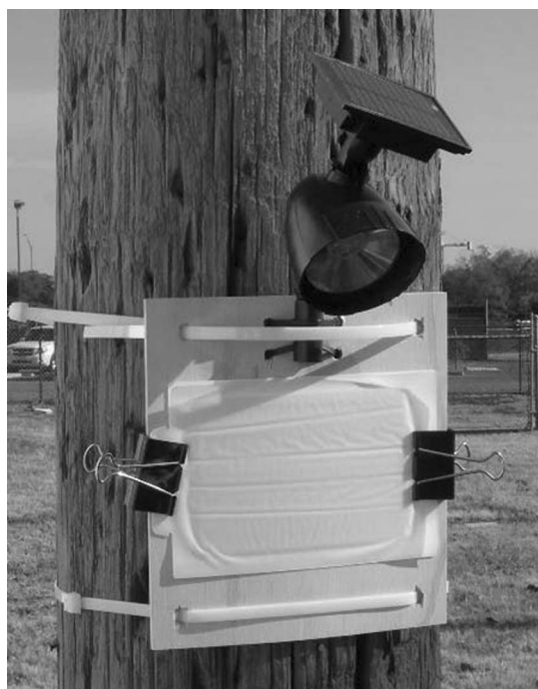
Fig. 1. C. formosanus alate trap with Hampton Bay solar LED spotlight and attached to a utility pole.
