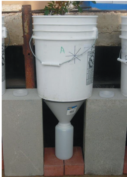
Fig. 1. Leachate was collected by placing a funnel inserted into a 1-liter Nalgene bottle under a bucket suspended by two hollow-block bricks.
