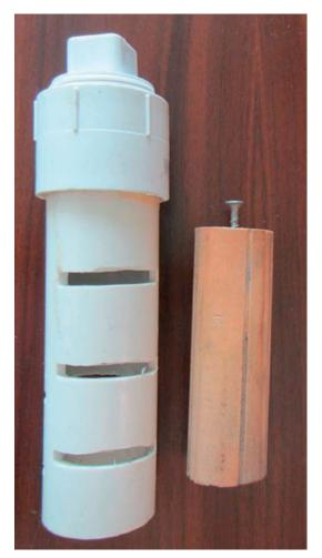
**Fig. 1.** Polyvinyl chloride (pvc) pipe (independent monitor [IM]) with southern yellow pine wood insert.
