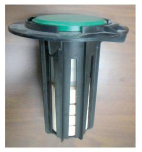
**Fig. 2.** Station with inspection cartridge with cellulose tablets and a monitoring base made of southern yellow pine.
